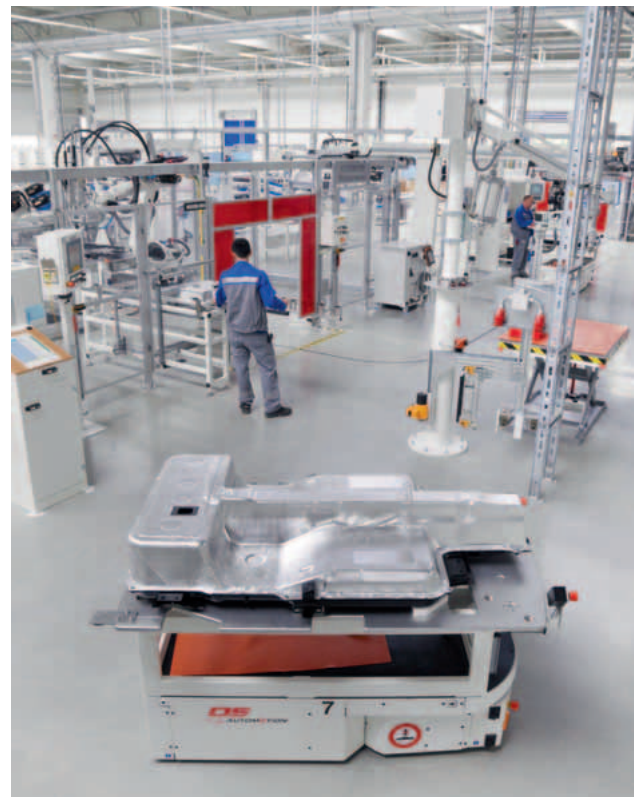
The battery systems for the e-up! are produced in-house in series in Brunswick. Forty employees produce 11,000 units per year.
