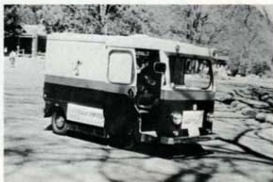
Lead-acid batteries provide the power for this van built by Electric Vehicles Inc.
