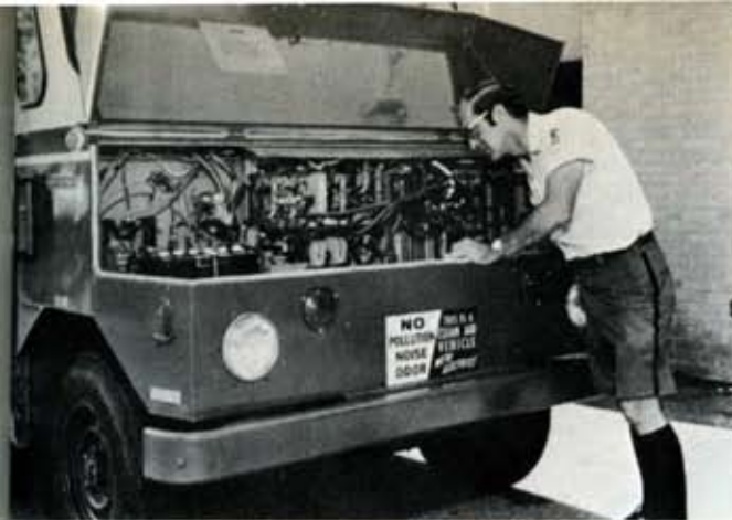
A look under the hood of an electric postal truck manufactured by Batronic Truck Corp.
