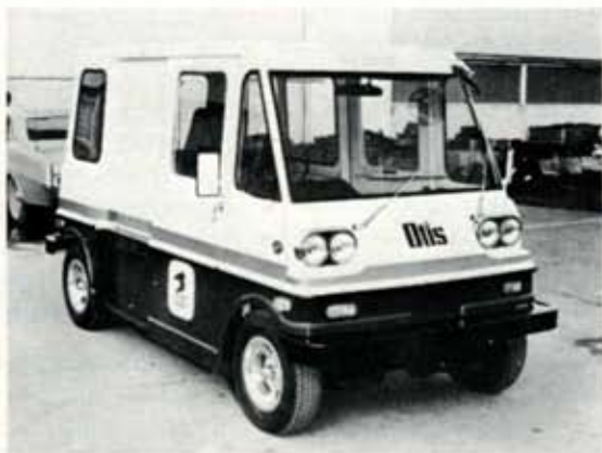
Otis Elevator Co. produced this van, now testing the feasibility of electric mail service vans at Santa Ana, Calif.
