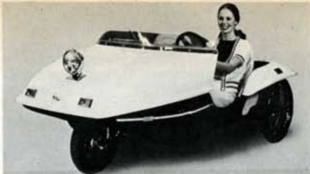
Battery-powered and capable of speeds in excess of 25 mph, this three-wheeler prototype was built by EVI Inc.
